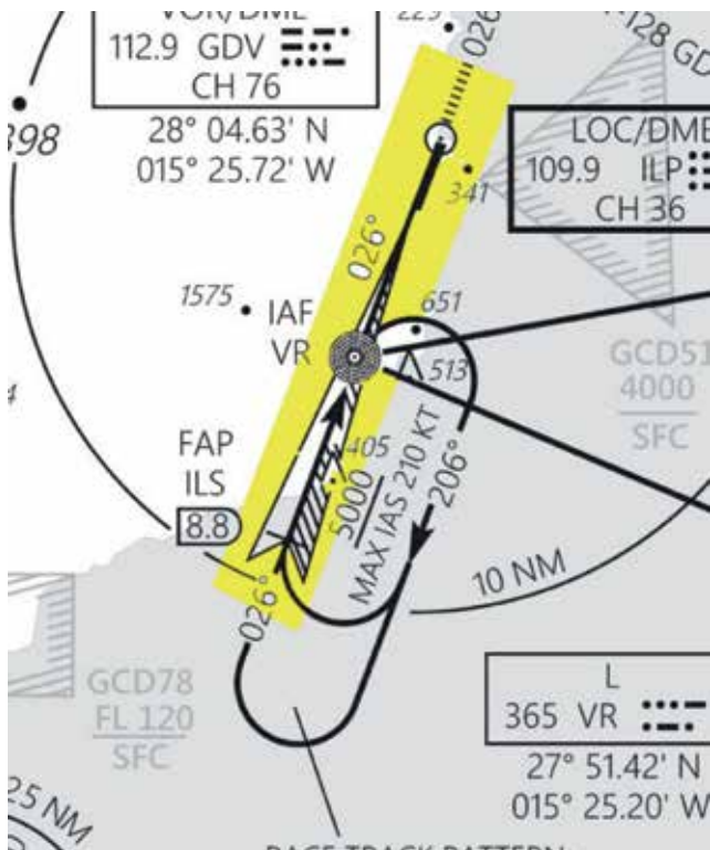
Figura 8. Instrumental Landing System (ILS)
