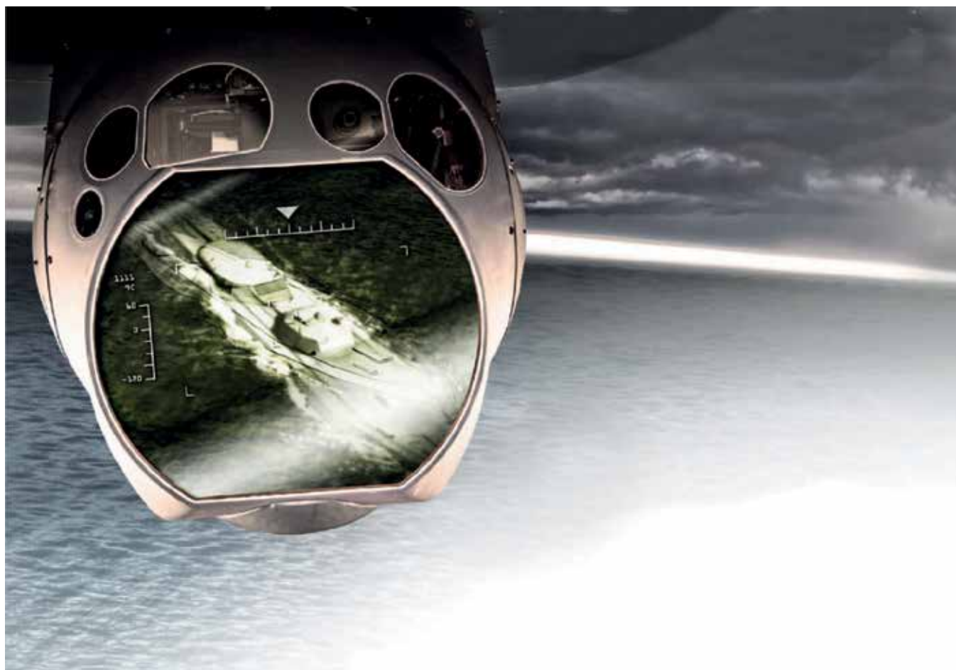
Figura 1. The Multi-Spectral Targeting System is a turreted electro-optical and infrared sensor used in maritime and overland intelligence, surveillance and reconnaissance missions. (Raytheon photo illustration created by Grant Parsley)
